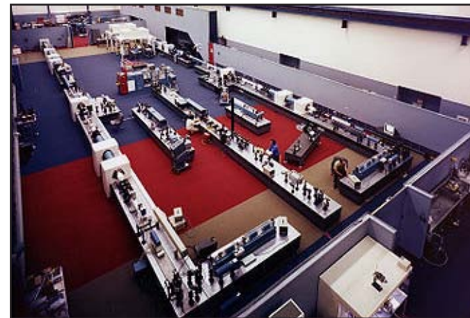
Argus – 2 beam, 2 kJ (LLNL) Nd:glass, 1 \mu\text{m} (1976)
