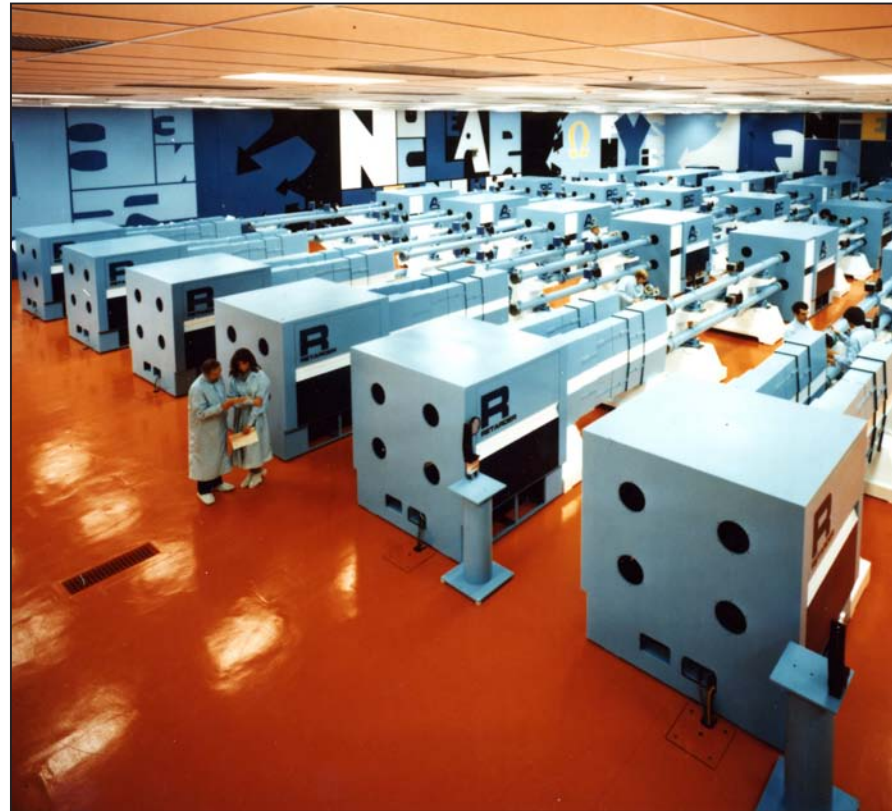
OMEGA – 24 beams, 4 kJ, 15 TW (LLE 1980)
