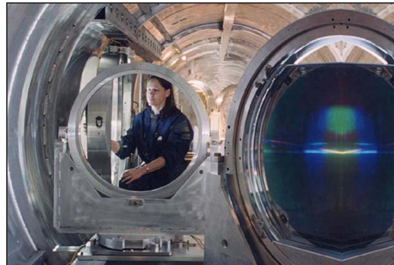
Grating chamber of the Nova PW
