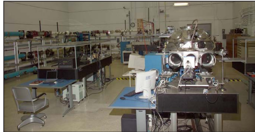
Pharos – 1 beam, 100 J, first disk amplifiers (NRL) Nd:glass, 1 \mu\text{m} (1971)
